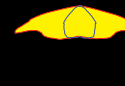
FS2 For symmetrical tunnel lighting and parking garages, ideal for catenary street lighting
