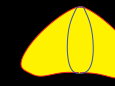
B2 / B2-STP For area lighting and applications demand- ing a wide oval beam pattern
