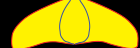
CAT-B ★ Narrow catenary street light beam optimized for EN13201 M-classes and tilted poles
