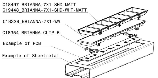
**Please Note:** If using C18354\_BRIANNA-CLIP-B, PCB needs seperate fixing to the housing for example screws.
