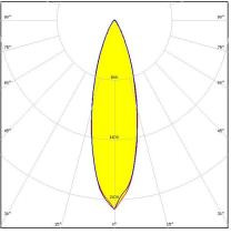
Dimensions: 35.0 mm x 35.0 mm Height: 8.52 mm ~24° medium beam
