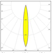
Dimensions: 35.0 mm x 35.0 mm Height: 8.52 mm ~18° spot beam
